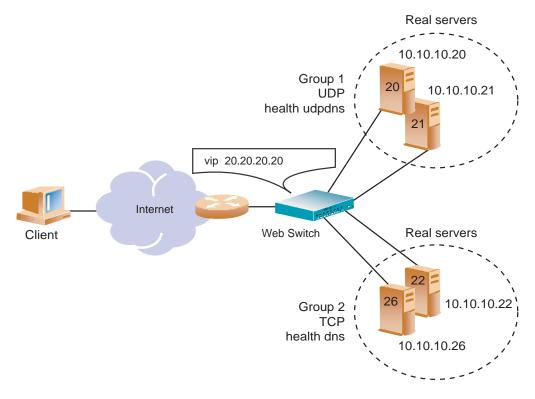
Figure 6-11 Layer 4 DNS Load Balancing
